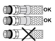
Before assembling the hose to the product ensure the hose ferrule has been crimped (as highlighted) on both ends of the hose after the braided hose sleeve.
